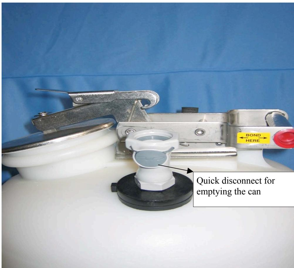
If your waste stream contains solids you will need a larger diameter tube to allow them to pass. We utilize a pass through fitting, which allows the tubing to penetrate the container when you are ready to extract the waste but is closed for transport to the processing area. An example of this follows:
