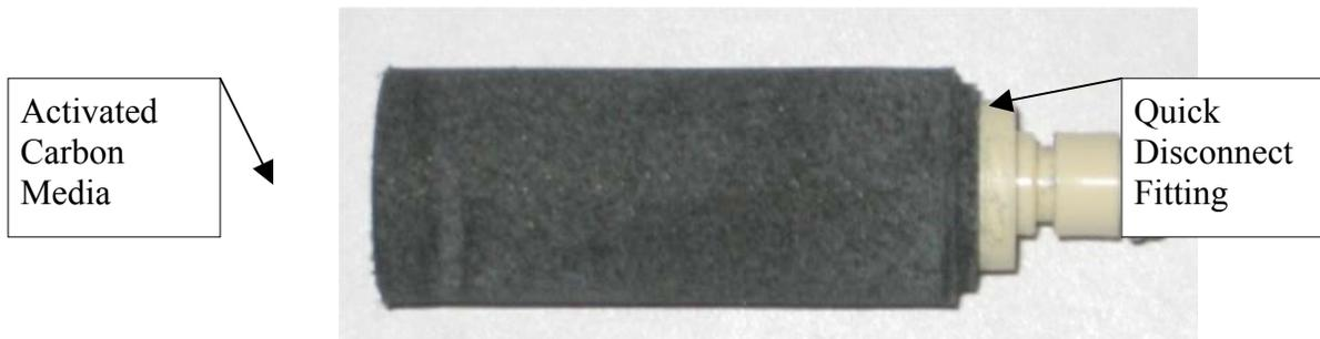
Directions for use: Insert the male quick disconnect fitting of the filter into quick disconnect female check valve on the safety can, connect the waste line into the other female check valve. When the container is full remove the filter and waste input line so that the container can be transported to the waste bulking area. The filter should be changed after two fillings of the container or when odors are detected.
