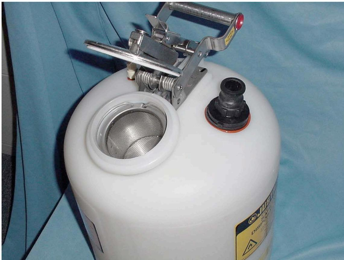
If the waste stream is coming from an HPLC, DNA synthesis or ink jet printer. We use quick disconnect fittings with check valves and an activated carbon filter vent. The purpose of the vent is to allow pressure to equalize with in the container. See below
