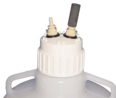
An activated carbon cartridge with a quick disconnect fitting designed for use with standard carboys and safety cans. Using this filter allows the pressure in the container to equalize when being filled from an HPLC machine while adsorbing the volatiles that are being released. The perfect solution to maintain air quality.
