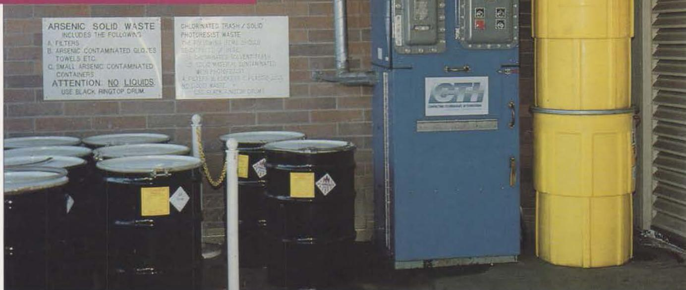
The manufacturing lines at USCI's facilities incorporate RCRA-listed solvents in the production process. The waste stream (wipes, filters, and towelettes), a flammable and hazardous waste, accounted for more than 60 percent of USCI's hazardous waste volume. After researching various methods of hazardous waste volume and cost reduction, in-drum compaction was identified as the most effective solution.
